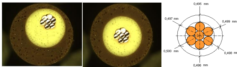
Fig. 1: Coating thickness geometry model
