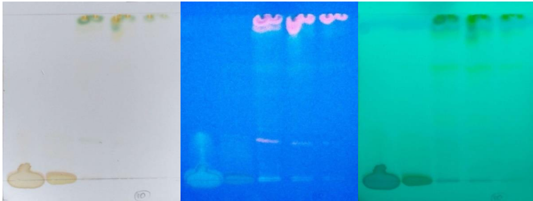
Fig. 3: developed TLC plates with stem extracts at visible range, 366nm and 254nm respectively.
