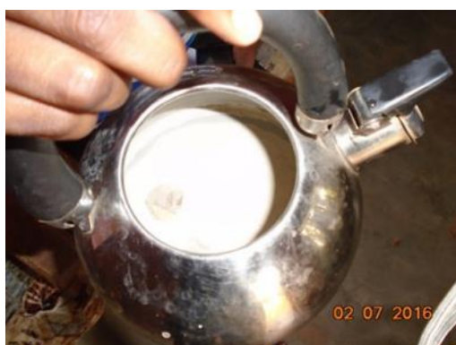
Fig. 5.7: Fluoride siltation inside a kettle after boiling the mineralized water (fluoride-rich water), Thanthirimale Source: Field survey (2016)
