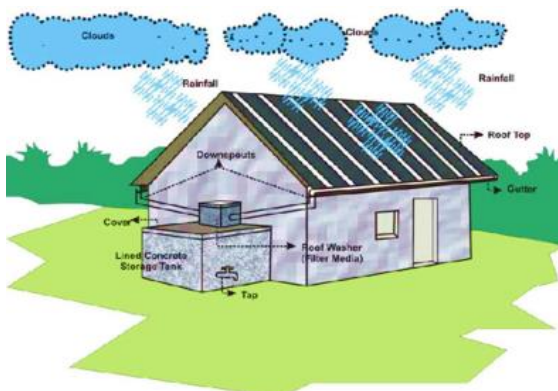
Fig. 5.1: Diagram of roof rain water harvesting system (above ground tank)
