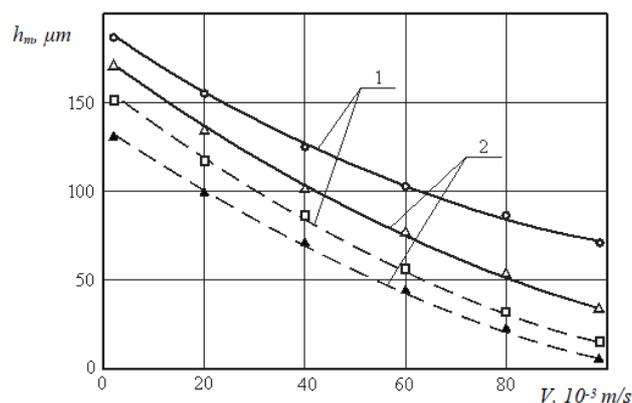
**Fig. 5:** The dependence of maximum thickness of melted layer in elements of optical glass BK10 (BK10) (1) and TF110 (ТФ110) (2) at  $F_n = 5 \cdot 10^8 \text{ Wt/m}^2$  (—) and  $F_n = 3 \cdot 10^8 \text{ Wt/m}^2$  (---) from travelling speed of electron stream ( $\Delta$ ,  $\circ$ ,  $\square$ ,  $\blacktriangle$  – experimental data).
