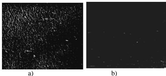
**Fig. 3:** Topogram of elements surface from optical glass BK-10 (BK-10): a) BK-10 glass surface after mechanical polishing,  $\times 2500$ ; b) BK-10 glass surface after treatment by electron flow,  $\times 2500$ .
