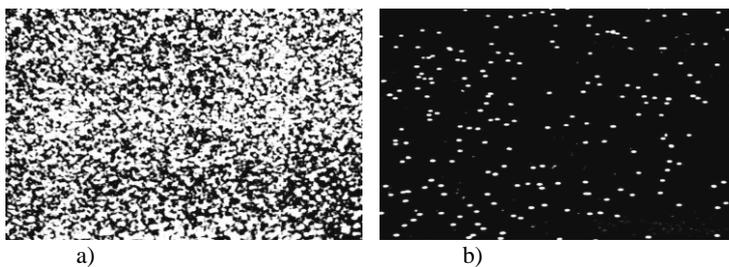
**Fig. 7:** Concentration distribution  $O_{\kappa\alpha}$  on the surface of elements from the optical glass K108: a) – before electron treatment; b) – after electron treatment.
