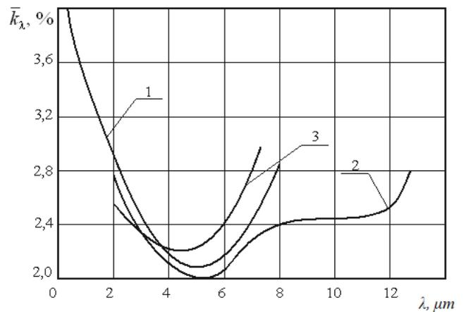
**Fig.15:** Dependence of relative coefficient of IR-radiation transmission of optical elements from ceramics KO5 (1), KO2 (2) и KO1 (3) (thickness of the flat layer of element  $H = 10^{-2} \text{ m}; T_0 = 300 \text{ K}; F_n = 1,5 \cdot 10^7 \text{ Wt/m}^2, V = 7 \cdot 10^{-3} \text{ m/s}$ ) from wave length.
