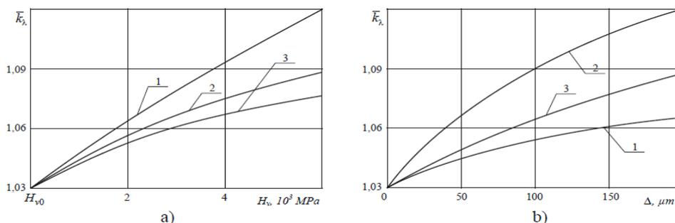
**Fig. 17:** Influence of microhardness of the surface  $H_v$  (a) and thickness of hardened layers  $\Delta$  (b) on the value  $\bar{k}_\lambda$  for the elements from optical ceramics KO5 (1), KO2 (2) и KO1 (3) ( $\lambda = 2 \mu\text{m}$ ).
