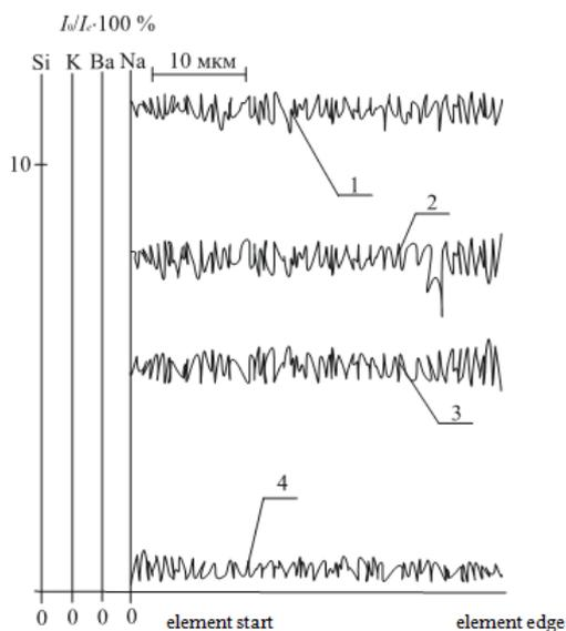
**Fig. 8:** Concentration distribution of elements on the surface of elements from optical glass BK10 (BK10) before electron treatment: 1 – Si, imp/sec; 2 – K·10<sup>3</sup>, imp/sec; 3 – Ba·10<sup>3</sup>, imp/sec; 4 – Na·10<sup>2</sup>, imp/sec.
