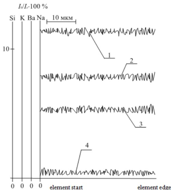
**Fig. 9:** Concentration distribution of elements on the surface of elements from optical glass BK10 (BK10) after electron treatment: 1 – Si, imp/sec; 2 – K·10<sup>3</sup>, imp/sec; 3 – Ba·10<sup>3</sup>, imp/sec; 4 – Na·10<sup>2</sup>, imp/sec.
