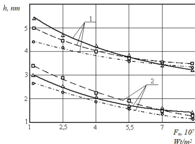
**Fig. 4:** Height dependence of residual microroughnesses on the surface of elements of optical glass K8 (—), TF110 (ТФ110) (---) and BK10 (BK10) (- · - ·) from the density of heat effect of electron beam for its different travel speeds:  $V = 5 \cdot 10^{-2}$  m/s (1);  $V = 8 \cdot 10^{-3}$  m/s (2) ( $\Delta$ ,  $\circ$ ,  $\square$  – experimental data).
