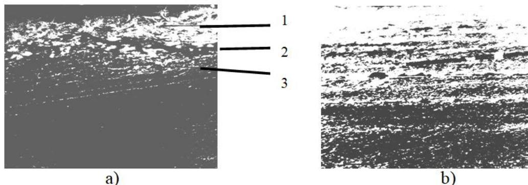
**Fig. 11:** Microstructure of etched section of chip of elements from optical ceramics KO2 after electron treatment: a – area of electron beam effect,  $\times 130$  (1 – plastic, 2 – space, 3 – affected area); b - area of electron beam effect,  $\times 350$ .
