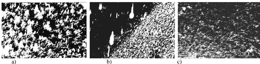
**Fig. 2:** Scans of the detail surface made of optical glass K208: a) K208 glass surface before electron-beam treatment, Y-modulation  $\times 610$ ; b) K208 glass surface at impact border electron-beam treatment, Y-modulation  $\times 122$ ; c) K208 glass surface after electron-beam treatment, Y-modulation  $\times 610$ .
