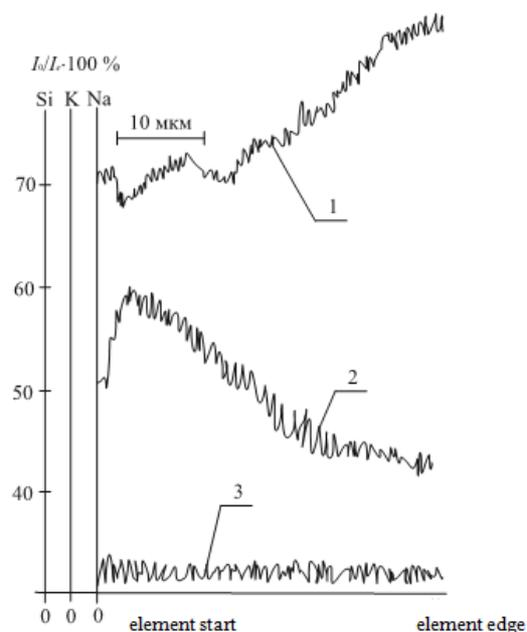
**Fig. 6:** Concentration distributions of elements on the surface of elements from the optical glass K108 after electronic treatment: 1 – Si·10<sup>4</sup>, imp/sec; 2 – Na·10<sup>3</sup>, imp/sec; 3 – K·10<sup>2</sup>, imp/sec.
