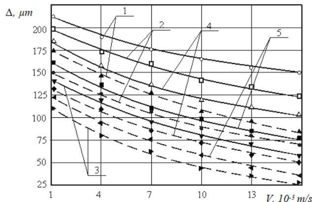
**Fig. 13:** Dependence of hardened layers of elements from optical ceramics KO12 (1), KO2 (2), KO1 (3), KO3 (4) and KO5 (5) at  $F_n = 1,5 \cdot 10^7 \text{ Wt/m}^2$  (—) and  $F_n = 2 \cdot 10^6 \text{ Wt/m}^2$  (---) from travel speed of electron beam ( $\Delta, \circ, \square, \blacktriangle, \blacksquare, \blacklozenge, \blacktriangledown, \bullet, \blacktriangleright, \blacktriangleleft$  – experimental data).
