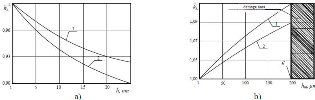
**Fig. 16:** Influence of residual microroughnesses  $h$  (a) and the thickness of melted layer  $h_m$  (b) on the value  $\bar{k}_\lambda$  for the elements from optical glass BK10 (1) and K8 (2) ( $\lambda = 1,06 \mu\text{m}$ ).
