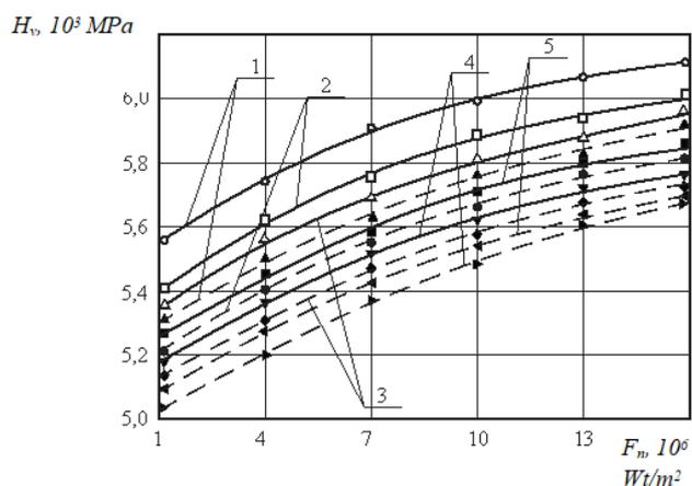
**Fig. 12:** Dependence of microhardness of elemental surface from optical ceramics KO12 (1), KO2 (2), KO1 (3), KO5 (4) и KO3 (5) at  $V = 7 \cdot 10^{-3} \text{ m/s}$  (—) and  $V = 1,5 \cdot 10^{-2} \text{ m/s}$  (---) from the density of thermal action of electron beam ( $\Delta, \circ, \square, \blacktriangle, \blacksquare, \blacklozenge, \blacktriangledown, \bullet, \blacktriangleright, \blacktriangleleft$  – experimental data).
