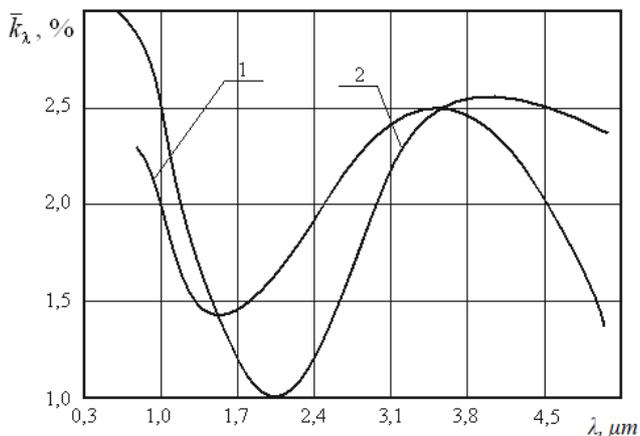
**Fig. 14:** Dependence of relative coefficient of IR-radiation transmission of optical elements from glasses K8 (1) and BK10 (2) (thickness of the flat layer of element  $H = 4 \cdot 10^{-3} \text{ m}; T_0 = 300 \text{ K}$ )
