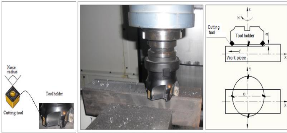
Fig. 5: Cutting tool and Tool holder of CNC Milling Operation
