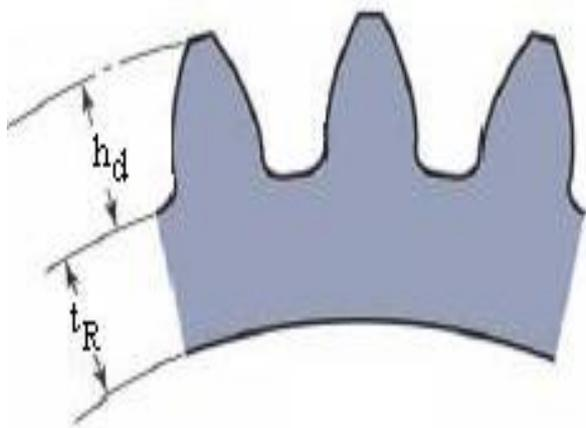
Fig.2: Rim Thickness and Whole Depth
