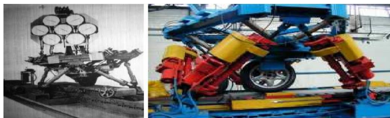
Fig.1: Gough Type Stewart Platform
