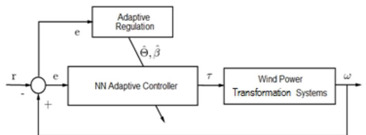
Fig. 1: Neural network adaptive controlled loops
