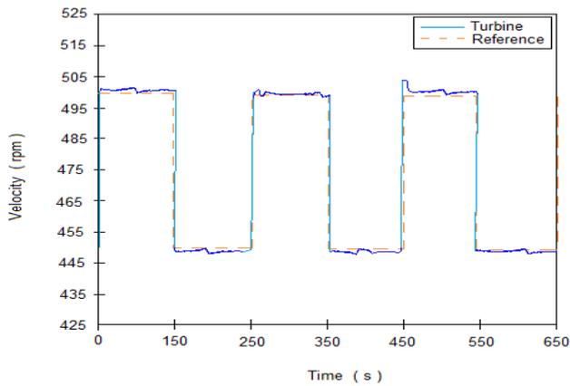
Fig. 2: Turbine velocity controlling performance
