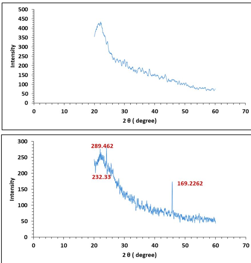
**Fig 3:** X-ray diffraction analysis (XR-D) study (a) Biosorbent citric acid modified tamarind pod shell unloaded with zinc (II) (b) Biosorbent citric acid modified tamarind pod shell with loaded with zinc (II)
