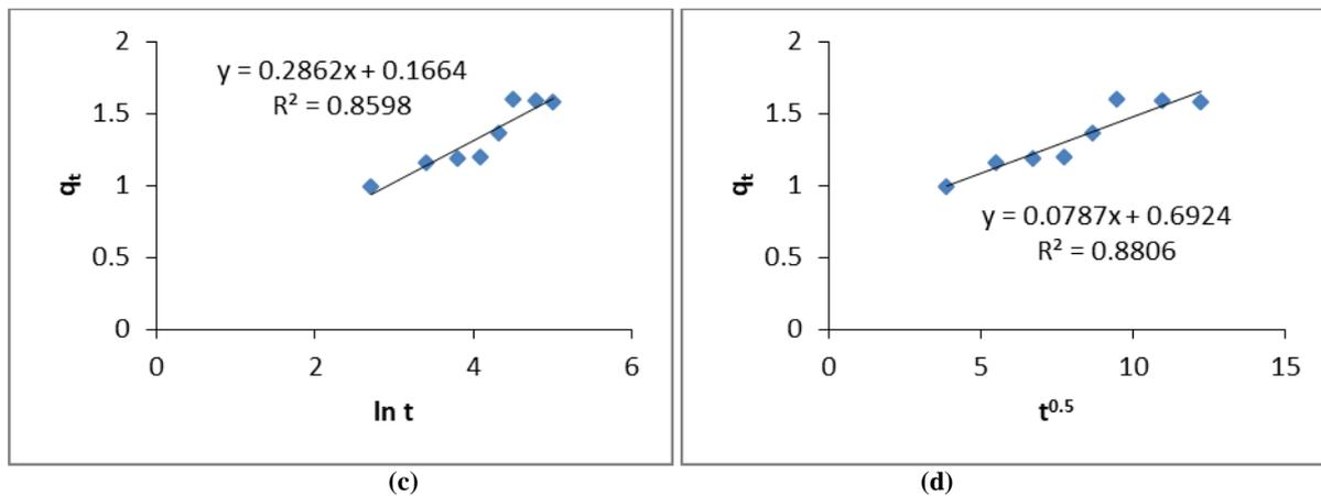
**Fig 11:** Adsorption kinetic models (a) pseudo-first-order, (b) pseudo-second-order (c) Elovich and (d) Weber and Morris intraparticle diffusion equation, for biosorption of zinc (II) citric acid modified tamarind pod shell (pH: 6.0, biosorbent dose concentration: 5 g/L, zinc (II) concentration: 5mg/L, temperature: 30°C, agitation rate: 120 rpm)
