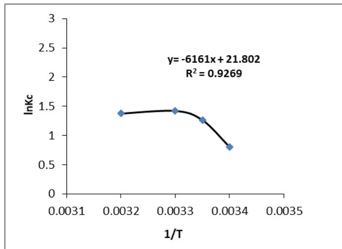
**Fig 12:** Plot of  $\ln K_c$  against  $1/T$  for determination of thermodynamic parameters for biosorption of zinc (II) by citric acid modified tamarind pod shell (pH: 6.0, biosorbent dose concentration: 5 g/L, initial zinc (II) concentration: 5 mg/L, agitation rate: 120 rpm contact time: 120 minute).
