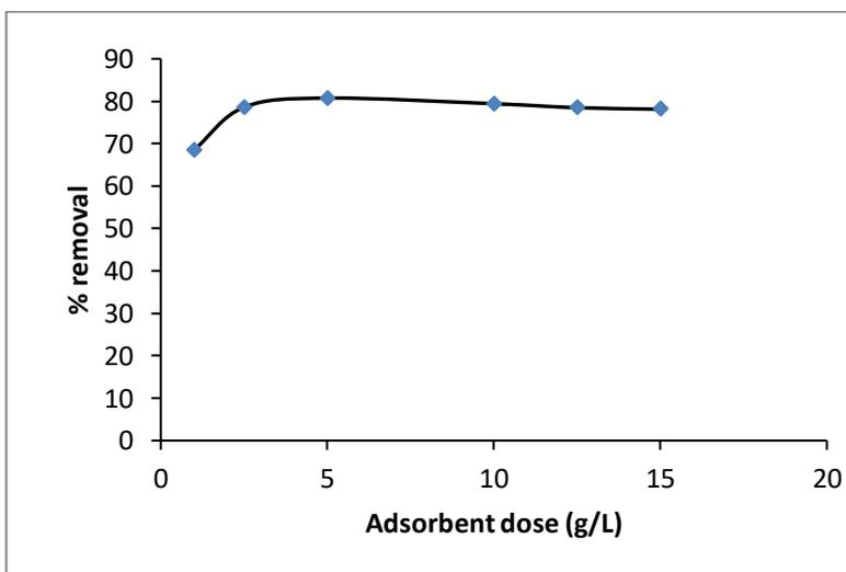
**Fig 5:** Effect of biosorbent dose concentration on zinc (II) biosorption citric acid modified tamarind pod shell (pH: 6, initial zinc (II) concentration: 5 mg/L, contact time: 120 minutes, agitation rate: 120 rpm, temperature: 30°C)
