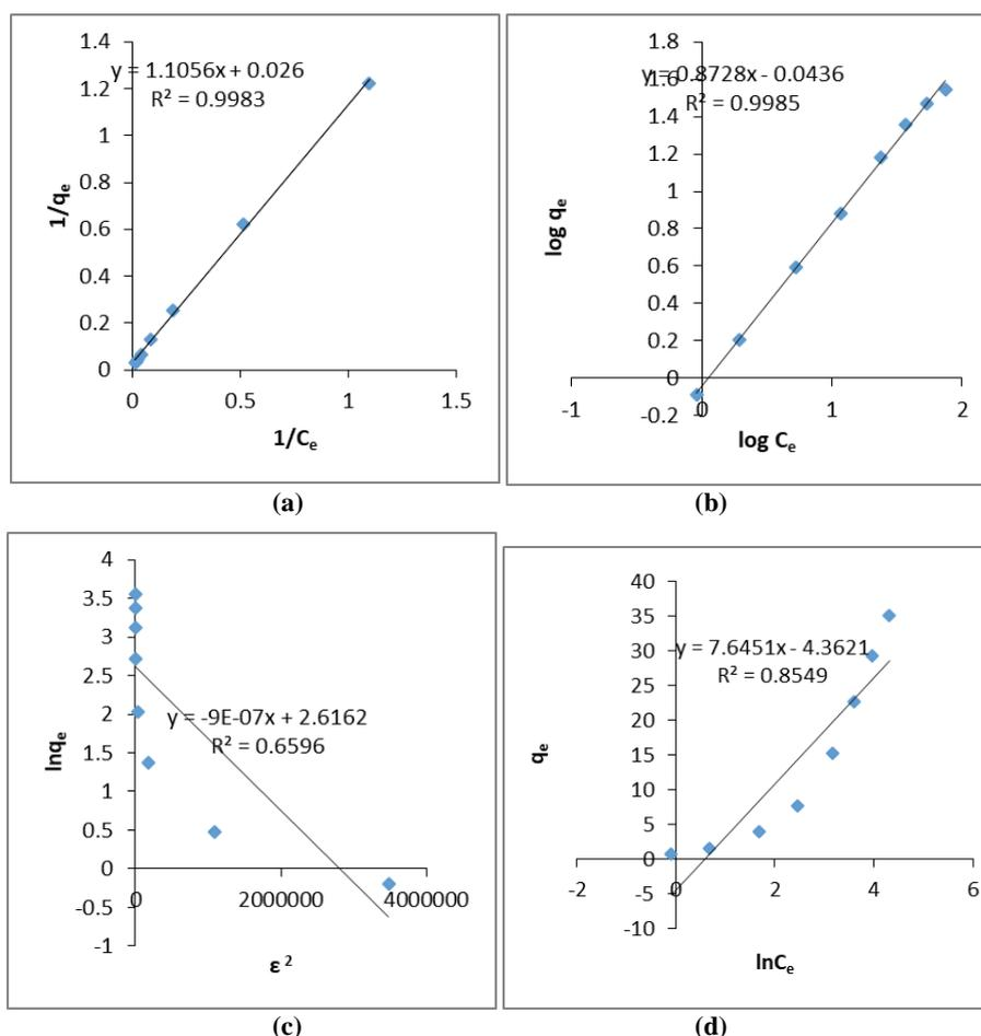
**Fig 10:** Adsorption isotherms (a) Langmuir, (b) Freundlich (c) DKR and (d) Temkin for biosorption of zinc (II) by citric acid modified tamarind pod shell (pH: 6.0, biosorbent dose concentration: 5 g/L, contact time: 120 minutes, temperature: 30°C, agitation rate: 120 rpm)
