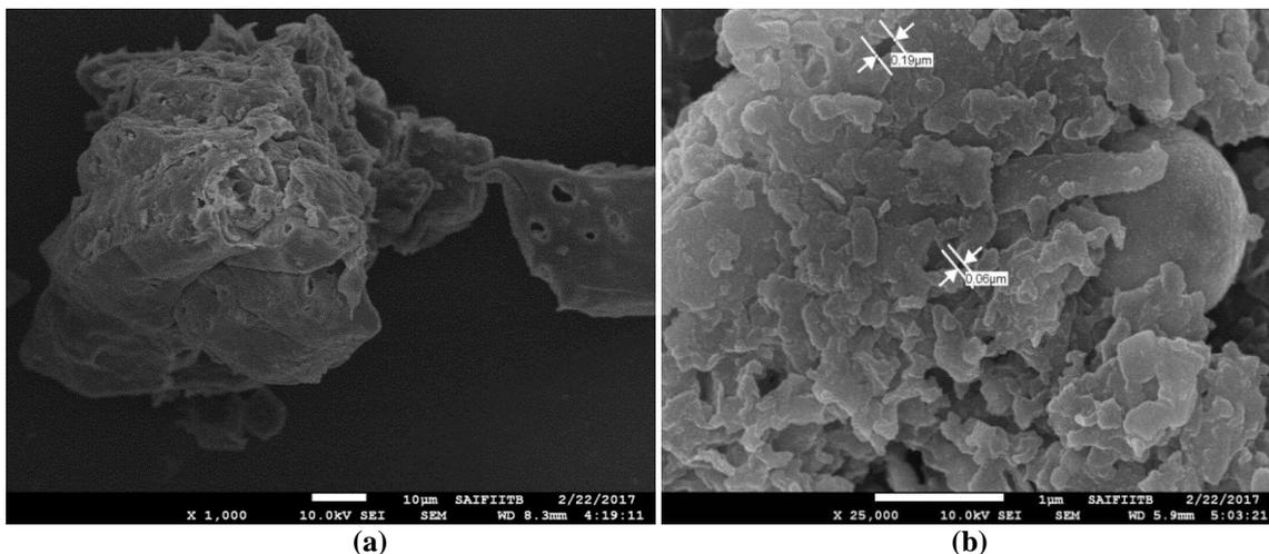
**Fig 2:** Scanning Electron Microscope (SEM) analysis (a) Biosorbent citric acid modified tamarind pod shell unloaded with zinc (II) (b) Biosorbent citric acid modified tamarind pod shell loaded with zinc (II)
