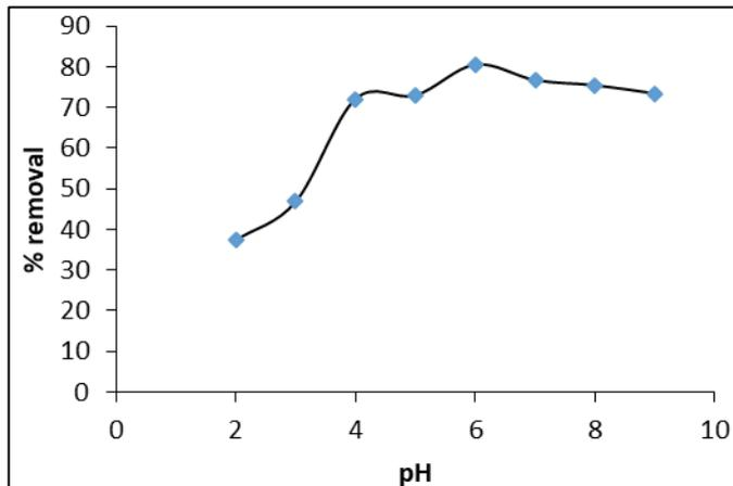
**Fig 4:** Effect of pH on zinc (II) biosorption by citric acid modified tamarind pod shell (Biosorbent dose concentration: 5 g/L, zinc (II) concentration: 5 mg/L, contact time: 120 minutes, temperature: 30°C, agitation rate: 120 rpm)
