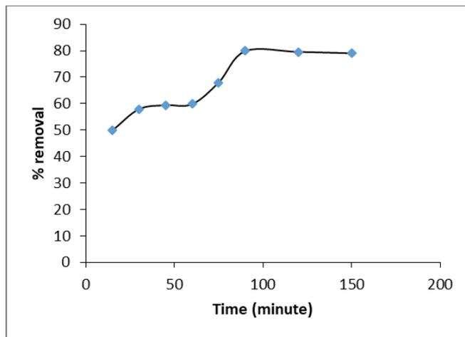
**Fig 6:** Effect of contact time on zinc (II) biosorption by citric acid modified tamarind pod shell (pH: 6, biosorbent dose concentration: 5 g/L, initial zinc (II) concentration: 5 mg/L, agitation rate: 120 rpm, temperature: 30°C)
