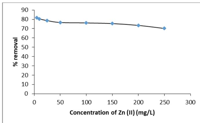
**Fig 7:** Effect of initial zinc (II) concentration on zinc (II) biosorption by citric acid modified tamarind pod shell (pH: 6, biosorbent dose concentration: 5 g/L, contact time: 120 minute, agitation rate: 120 rpm, temperature: 30°C)
