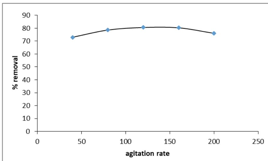
**Fig 9:** Effect of agitation rate on zinc (II) biosorption by citric acid modified tamarind pod shell (pH: 6, biosorbent dose concentration: 5 g/L, initial zinc (II) concentration: 5 mg/L, contact time: 120 minute, temperature: 30°C)
