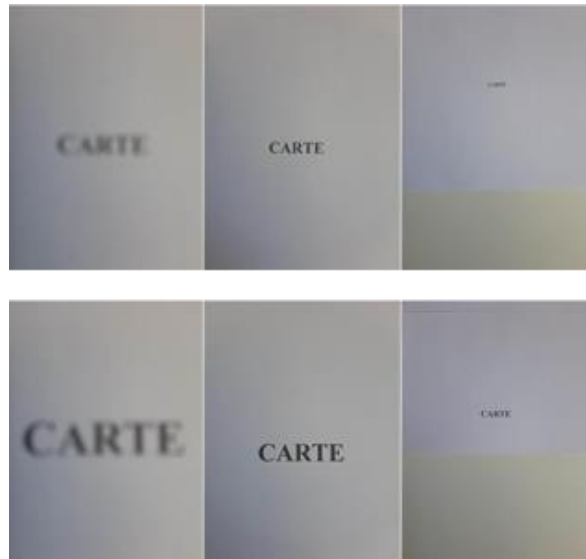
Fig. 5: UP - Word "CARTE" (book) at distances of 2, 4 and 12 cm with a font size of 12 DOWN - Word "CARTE" (book) at distances of 2, 4 and 12 cm with a font size of 26
