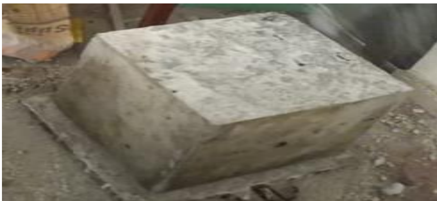
Fig. 4: Demoulded concrete ready for curing.
