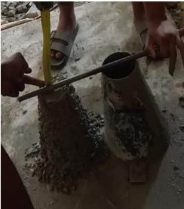
Fig. 2: Slump test for 20% replacement.
