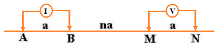
Fig. 2: Dipole-dipole electrode Array
