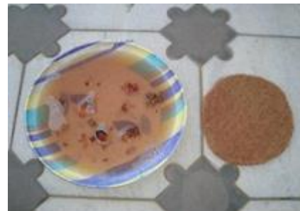
Fig.2: Dissolved Glue with Coir Sample
