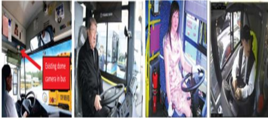
Fig.1: Existing dome camera in the bus and example images of bus drivers captured by the dome cameras in buses. Only an oblique view of low-resolution face images can be captured by the existing dome cameras for normal driving poses. (Images came from open sources of bus service companies with face portions of the drivers being pixelated for keeping anonymity.)[1]
