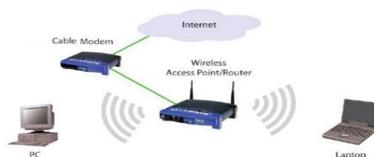
Fig. 1.1: A Simple Wireless network [3]
