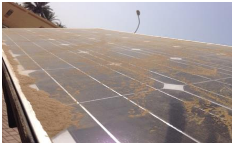
Fig. 1: the tested PV cell after being loaded by 300 gr of dust
