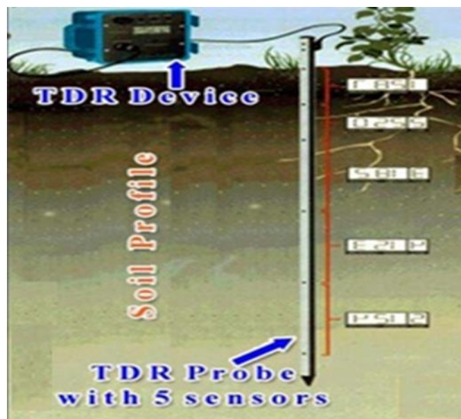
Fig. 3: TDR device and probe with five sensors.
