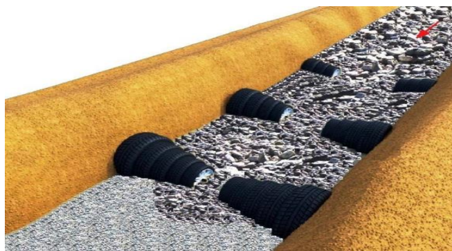
Fig. 1: Penetrating type of anti-debris flow structure.
