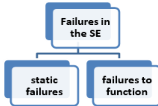
Fig.1. Failures in the switching equipment
