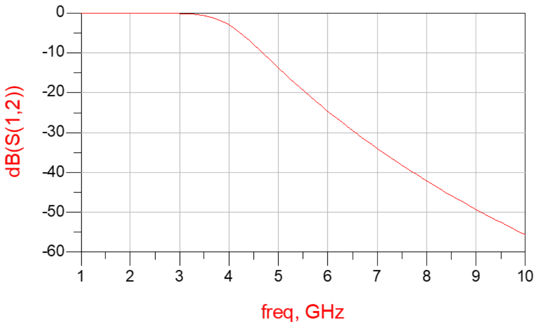
Fig. 6: The characteristic of the microwave filter showing variation of incident wave with frequency.
