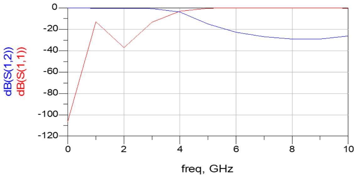
Fig. 23: The characteristic of the distributed transmission line showing variation of both incident wave and the forward gain with frequency.
