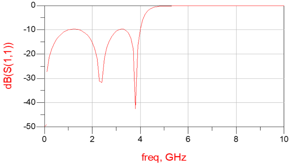
Fig. 14: The characteristic of the chebyshev filter showing variation of incident wave with frequency.
