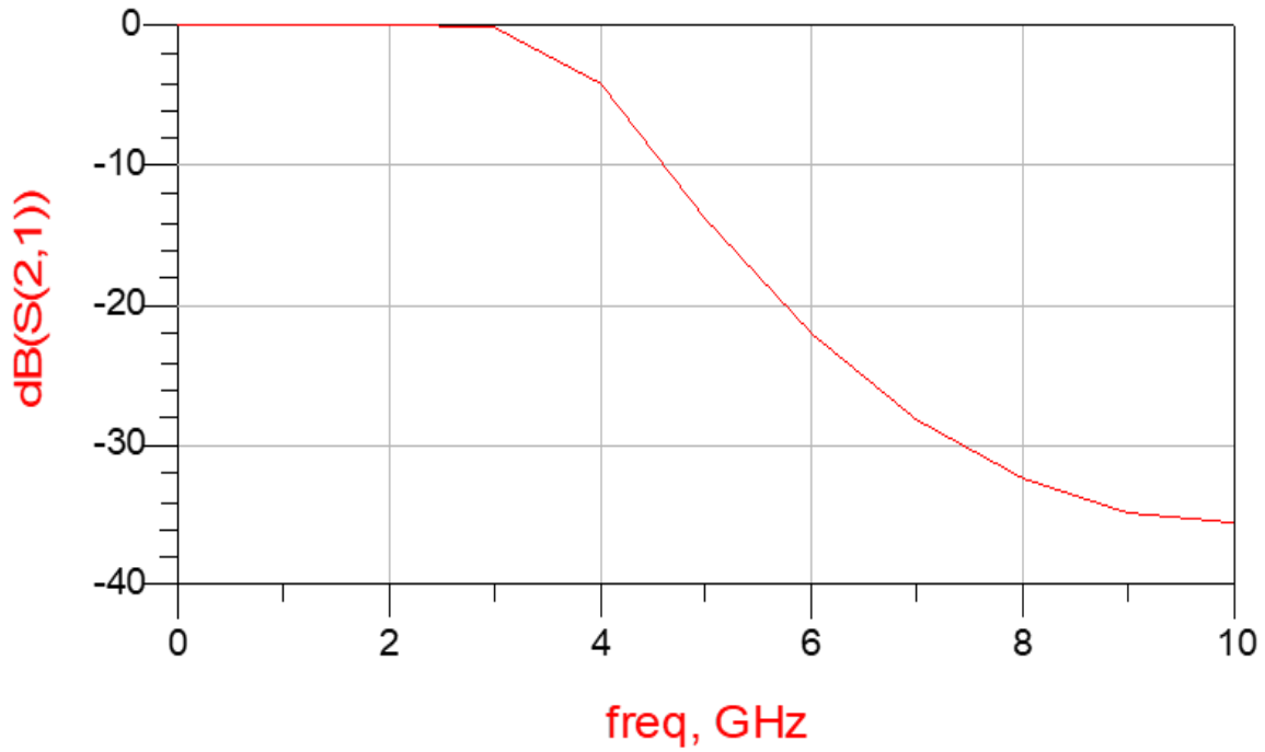
Fig. 12: The characteristic of distributed transmission line showing variation of reversed gain with frequency
