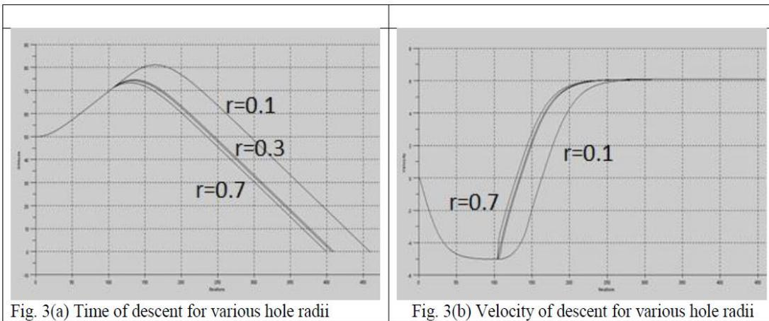
Fig. 3(a) Time of descent for various hole radii
