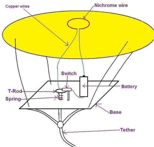
Fig. 1: Schematic diagram of Payload Recovery Device (PRD) [2]
