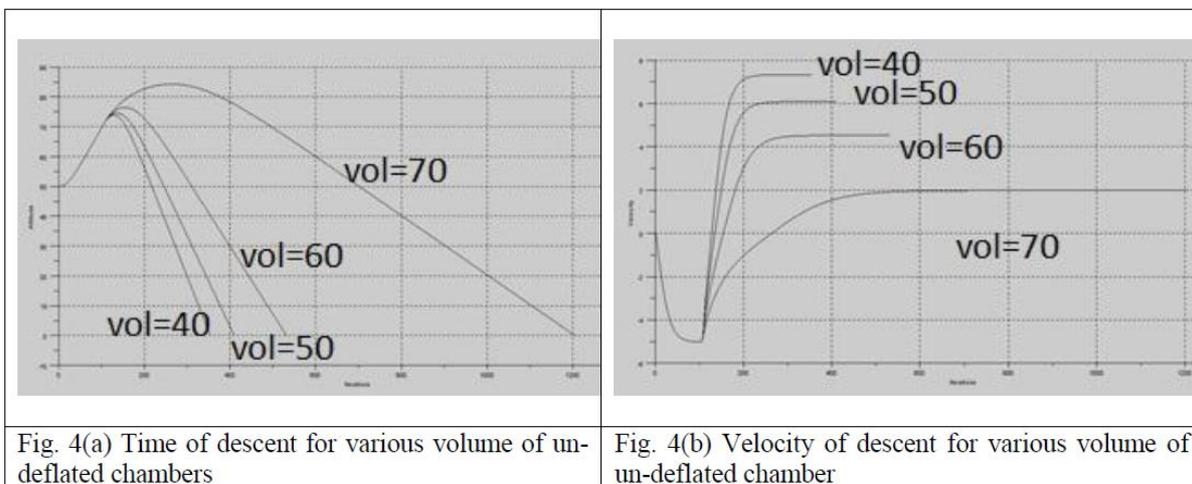
Fig. 4(a) Time of descent for various volume of un-deflated chambers
