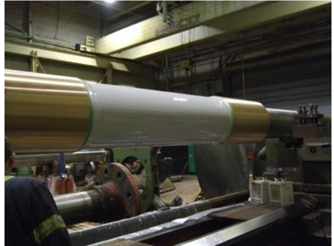
Fig. 5: Bearing of crankshaft based on BSn5Zn5Pb5
