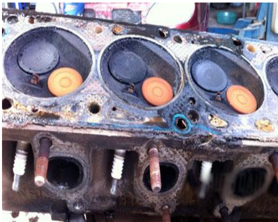
Image 4: Diesel engine corrosion
