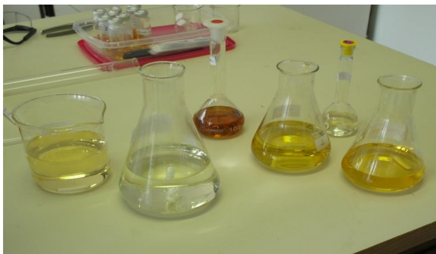
Fig 2: Different protic ionic liquids used in this work as catalysts for triacetin synthesis by esterification of glycerol
