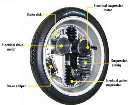
Fig. 2: Michelin active tire with in-wheel electric motor.
