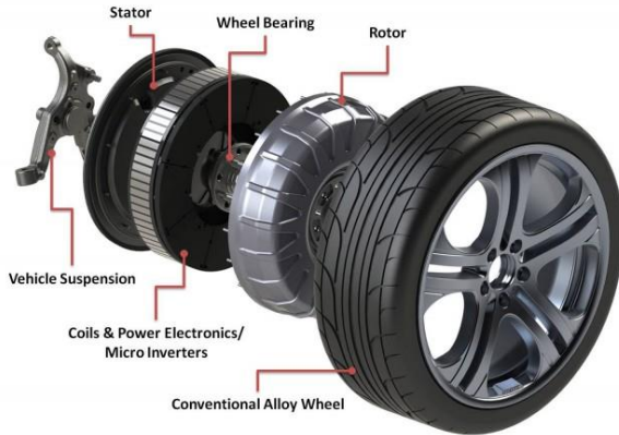
Fig. 1: In-wheel electric motor system.
