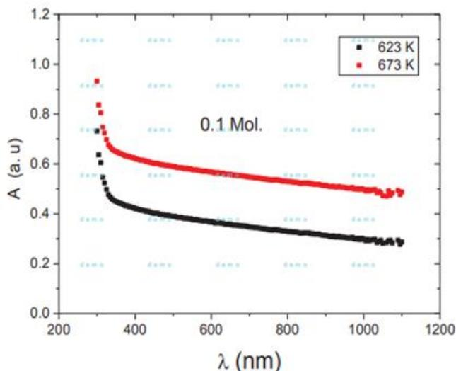
**Fig. 3:** UV -vis absorbance (A) spectra of CdO thin films deposited at different annealing temperature.
