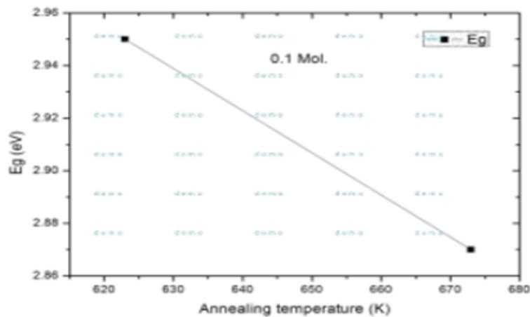
Fig. 9: Variation of energy gap with annealing temperature.
