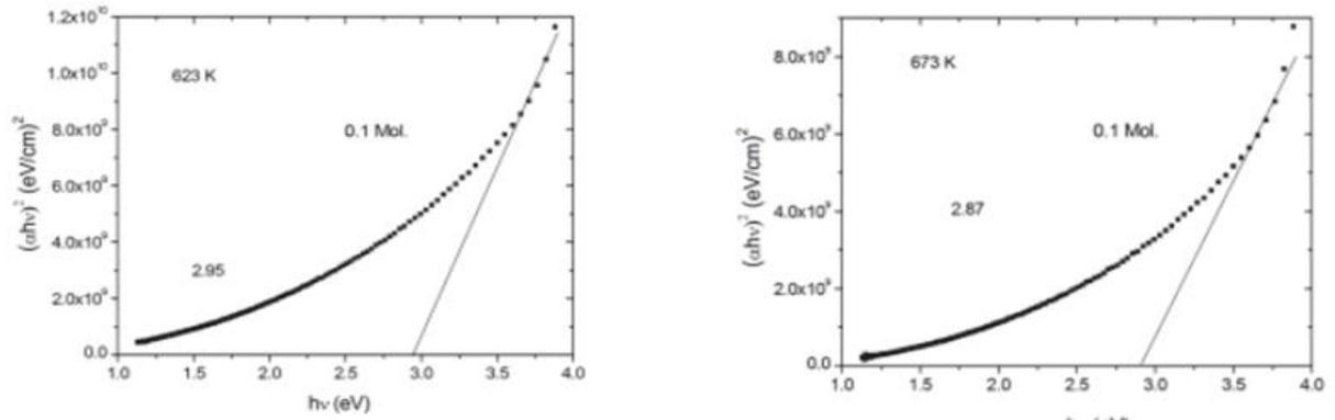
Fig. 7: A direct band gap of CdO thin film deposited at different annealing temperature.
