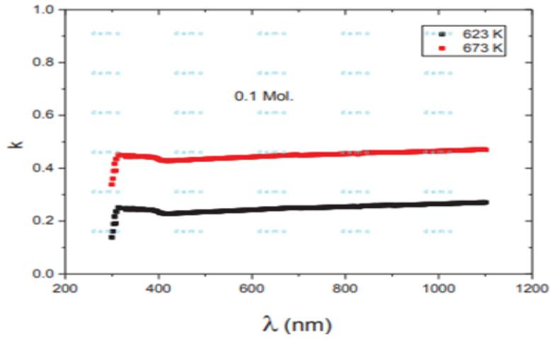
Fig. 6: Extinction coefficient (k) as a function of wavelength ( $\lambda$ ) for CdO thin films deposited at different annealing temperature.
