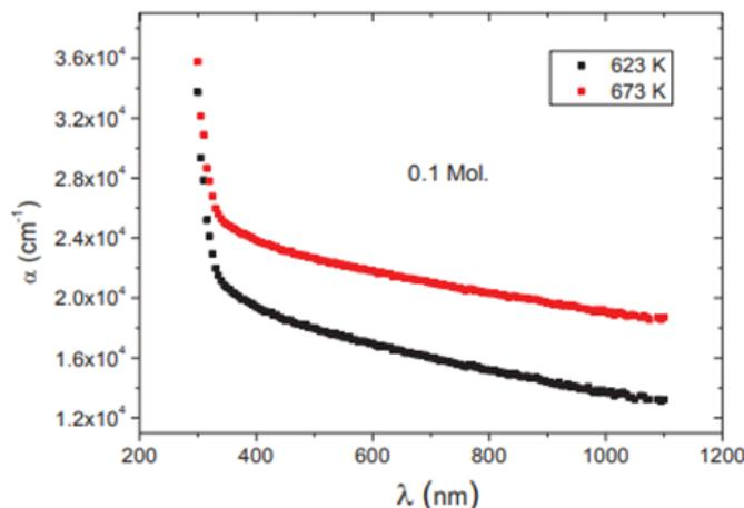
**Fig. 5:** Absorption coefficient ( $\alpha$ ) as a function of wavelength ( $\lambda$ ) deposited at different annealing temperature.
