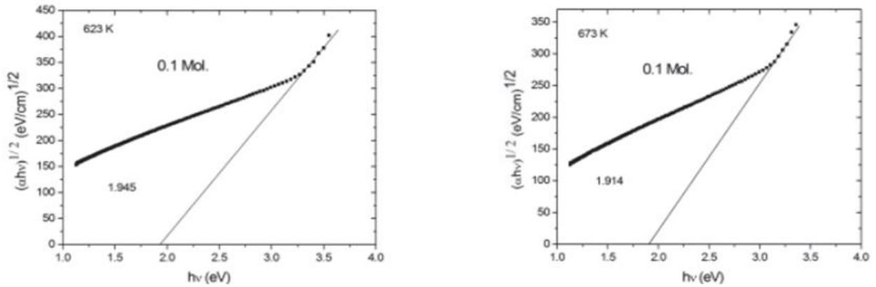
Fig. 8: An indirect band gap of CdO thin film deposited at different annealing temperature.
