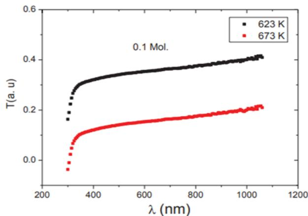
**Fig. 4:** UV -vis Transmittance (T) spectra of CdO thin films deposited at different annealing temperature.
