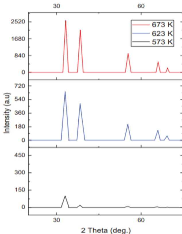
**Fig. 1:** XRD pattern for annealed CdO thin film at different annealing temperature.
